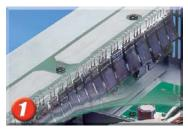
Amplifier reliability depends on reducing stress on transistor output devices. The Black Max uses **14 large output transistors** per channel for the utmost in high reliability.
